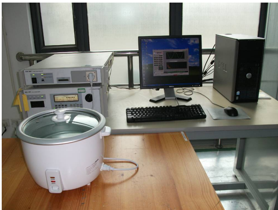
Figure B-4 Setup for Harmonic current emission and Voltage fluctuations and flicker
