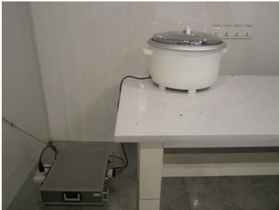
Figure B-5 Setup for conducted emission
