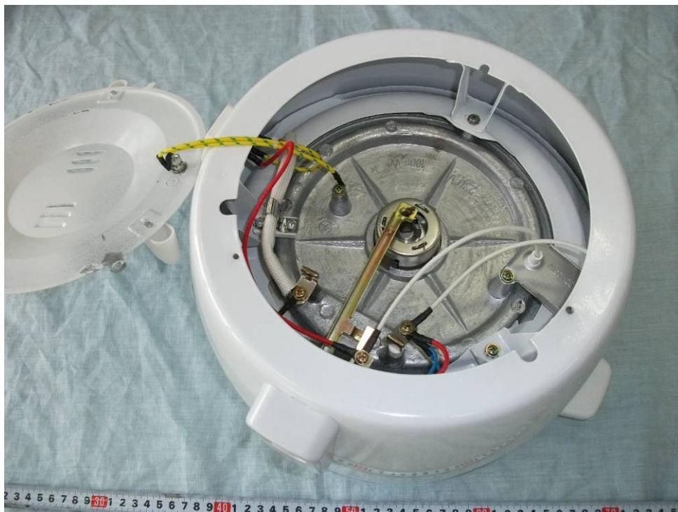
Figure A-5 Electrical Circuit Photo of RC-16A
